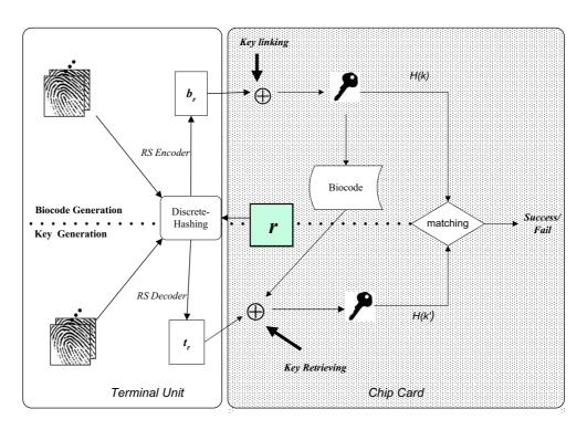
Figure 1: Application-specific key release scheme
