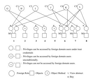
Figure 5: An example of ORBAC object diagram in multiple secure domains
