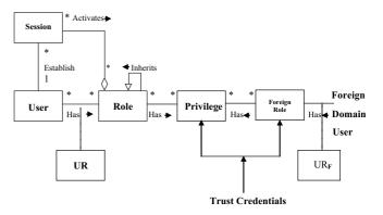
Figure 4: Class diagram of ORBAC model for multiple secure domain environment
