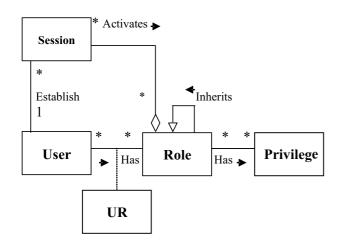
Figure 1: Class diagram of ORBAC model for single secure domain environment
