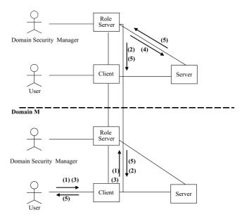
Figure 8: Collaboration diagram for multiple secure domain management architecture
