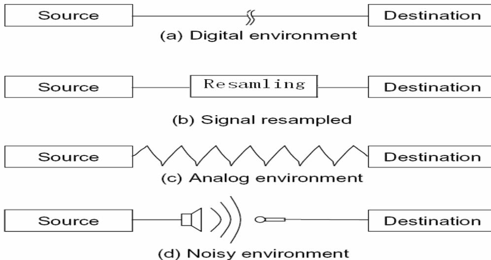
Figure 1: Transmission environments of digital audio [15]
