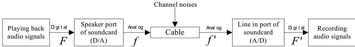
Figure 2: Test Model for DA/AD
