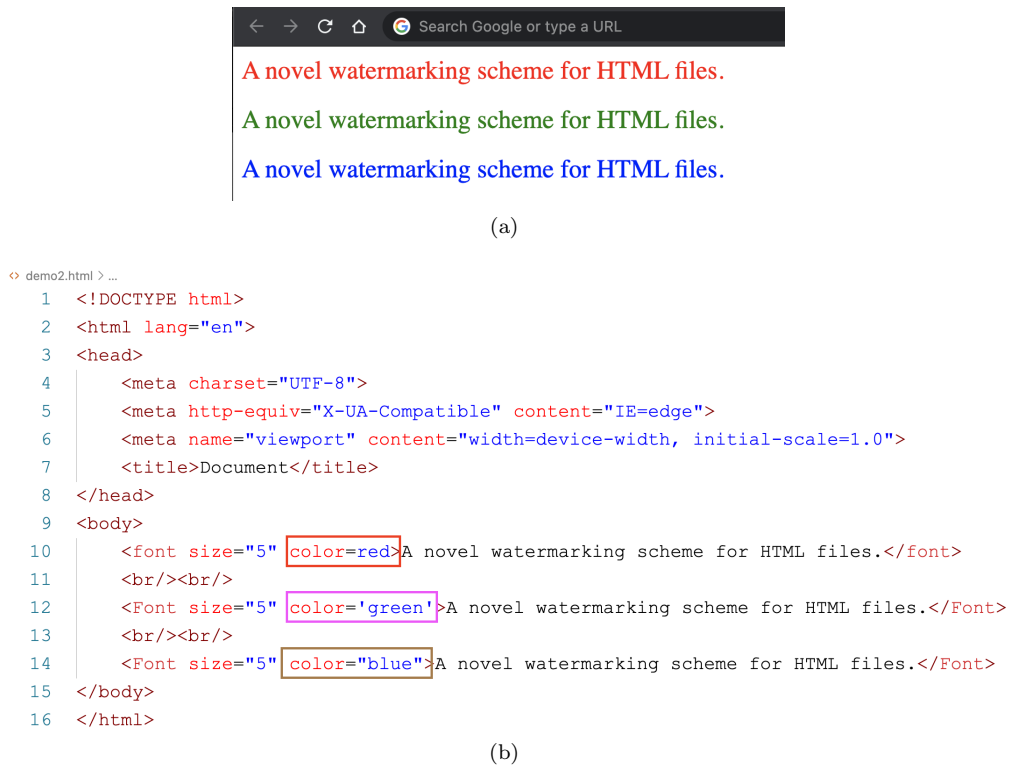
Figure 3: An illustration of Yang and Yang method [17]. (a) The result of using different "quotation marks" in the color attribute of the <font> tag. (b) Source code of Figure 3(a).
