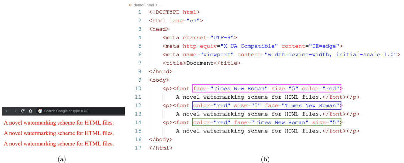
Figure 4: An illustration of Huang et al. data hiding method [11, 12]. (a) Results are presented in different order of attributes. (b) Source code of Figure 4(a).
