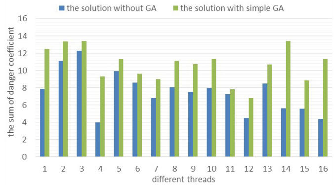
Figure 7: The differences in the sum of danger coefficient between using GA and not using GA
