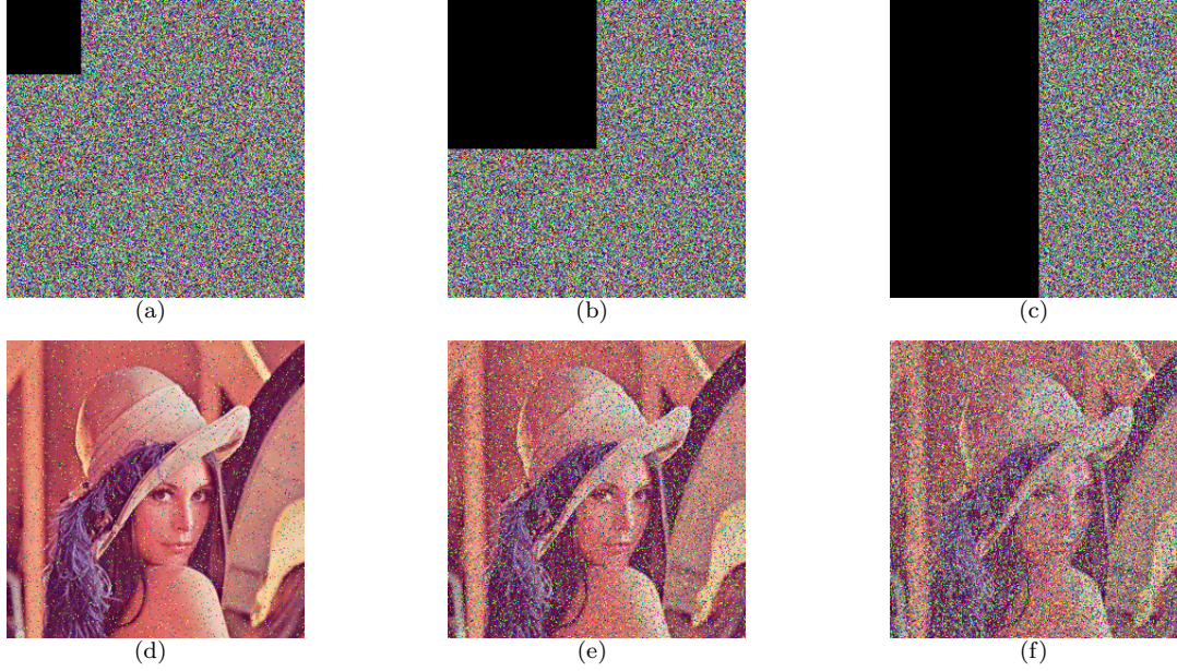
Figure 6: The encrypted Lena with (a) 1/16, (b) 1/4, (c) 1/2 data cropping; corresponding decrypted images (d)-(f) from (a)-(c).
