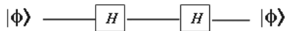
Figure 6: Two Hadamard gates in series restore a qubit to its original state
