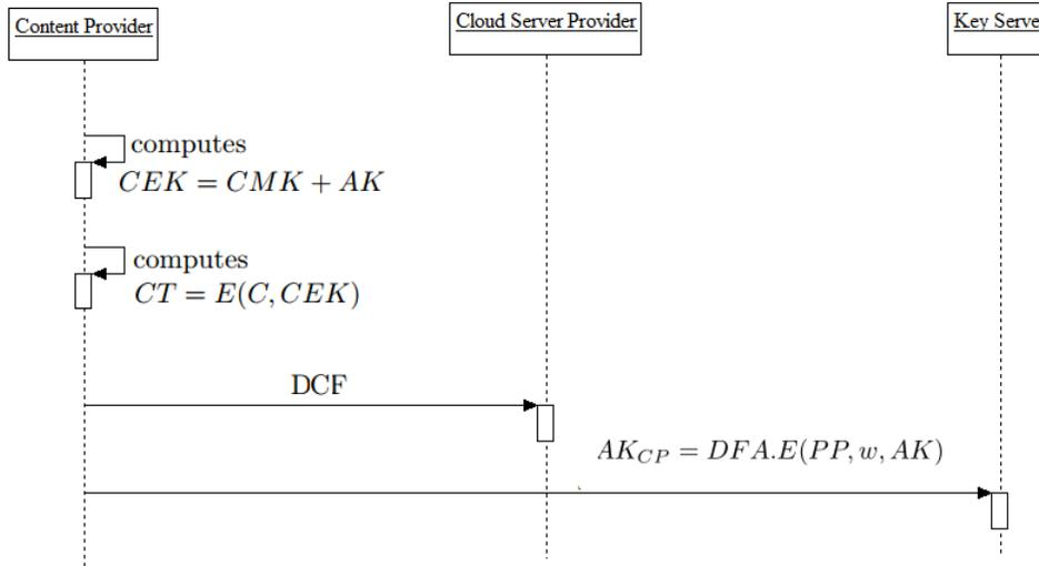
Figure 2: The sequence diagram of content encryption steps
