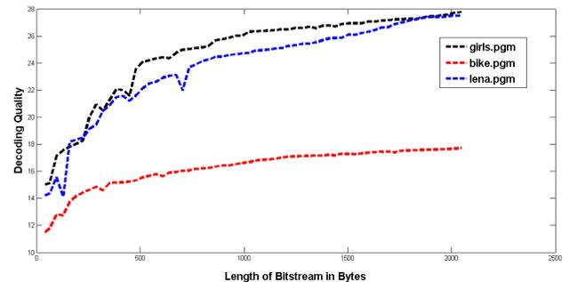
Figure 2: Decompression quality change within the first 2048 bytes
