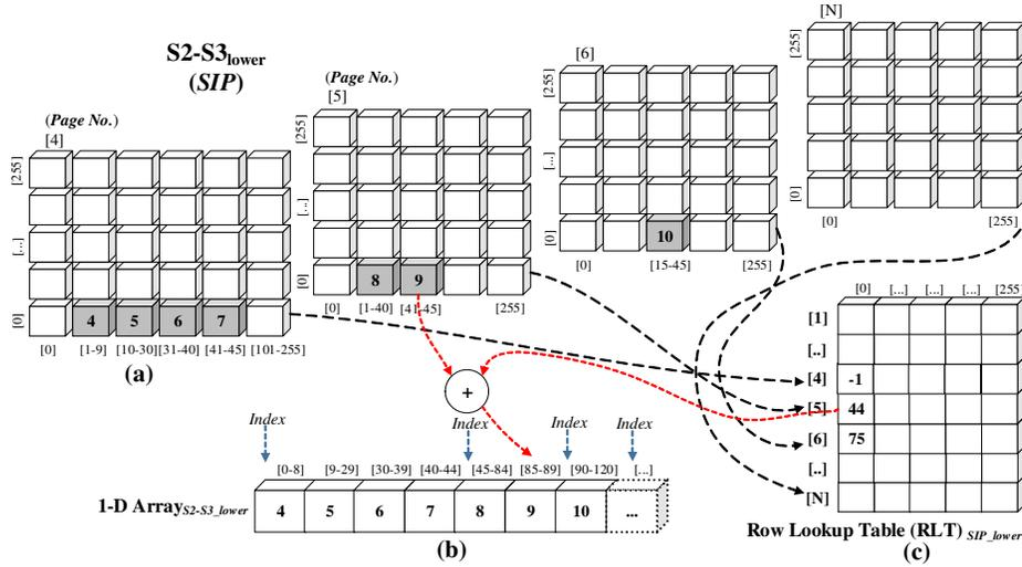
Figure 9: (a) separating the 3-D array of  $SIP$  namely  $S2-S3_{lower}$  to records, (b) packing records to 1-D array, and (c) adding the starting position of each packed record to RLT
