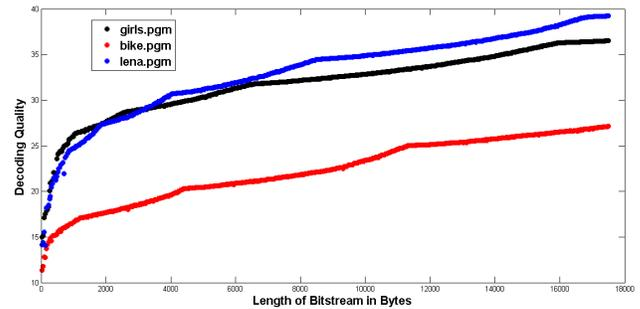
Figure 1: Decompression quality change through the whole bitstream
