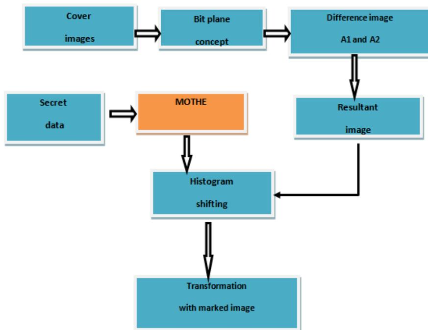
Figure 1: Encryption scheme
