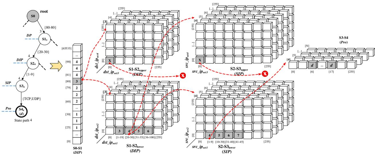
Figure 8: Mapping the 4<sup>th</sup> state path of DSD to array structures
