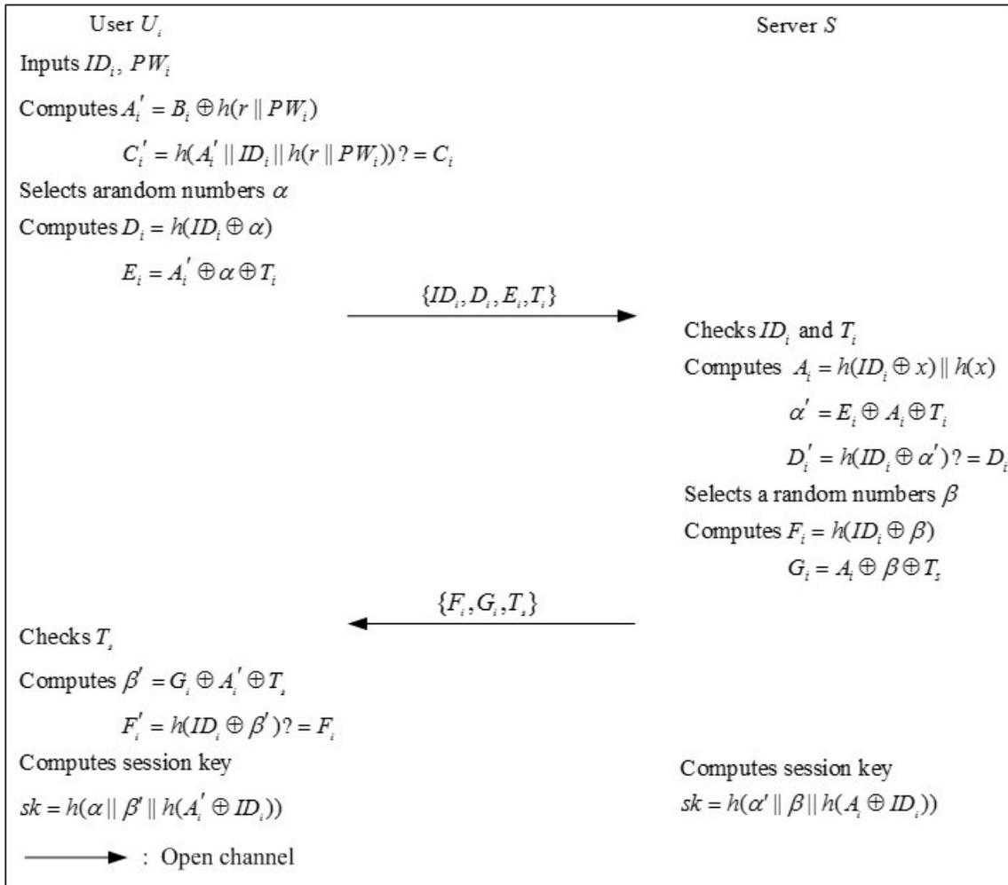
Figure 3: Login and authentication phases of our proposed scheme
