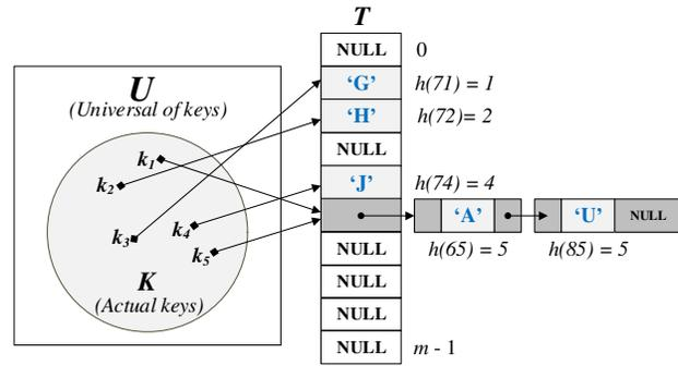
Figure 2: Five hash values  $h(k_1), \dots, h(k_5)$  in hash table
