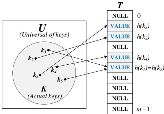
Figure 1: Using hash function ( $h$ ) maps actual keys with values to hash-table slots
