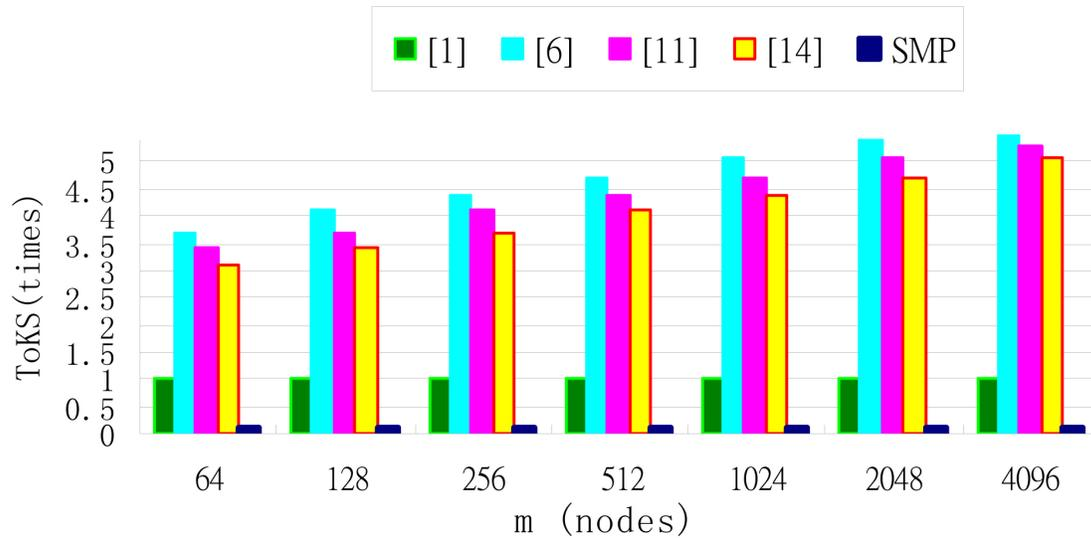
Figure 7: Key storage cost vs.  $m, d = 4$
