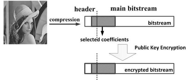
Figure 4: Proposed asymmetric encryption model-encryption process
