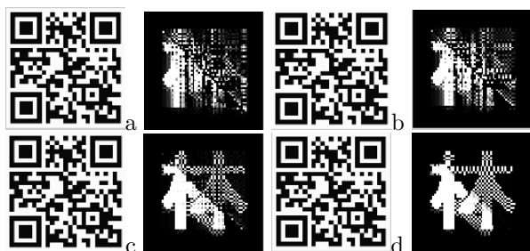
Figure 7: Watermark barcode with different embedding factor and extracted watermark: (a) Embedded factor 0.1; (b) Embedded factor 0.05; (c) Embedded factor 0.01; (d) Embedded factor 0.001
