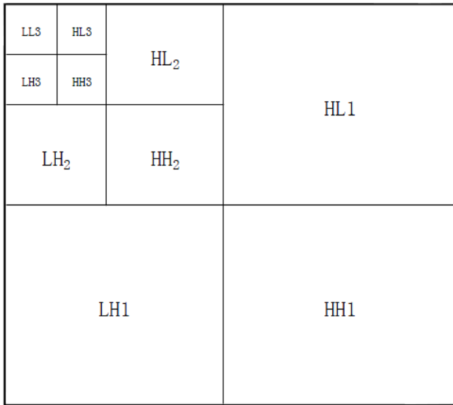
Figure 2: Decomposition diagram based on DWT
