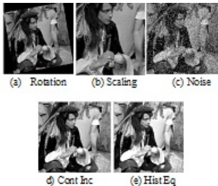
Figure 7: Cover image man embedded with CS logo watermark with various attacks a) Noise, b) Rotation, c) Cont Inc, d) Hist Eq, e)Scaling
