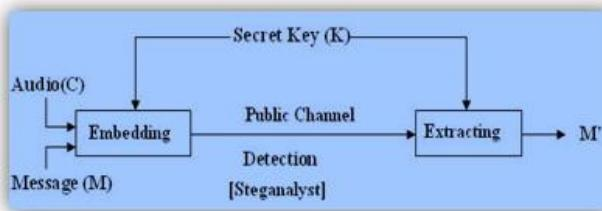
Figure 1: Basic data hiding process
