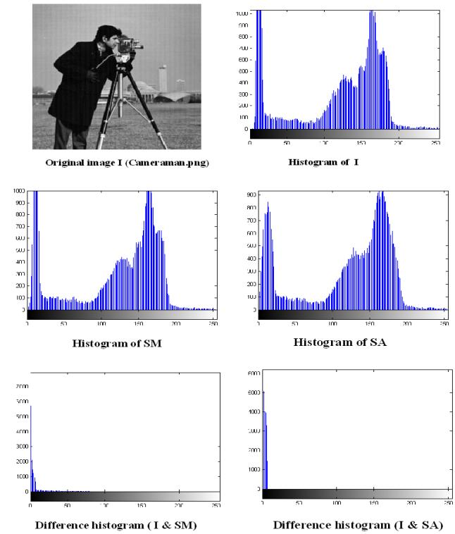
Figure 7: Histogram of Original, SM, SA and difference
