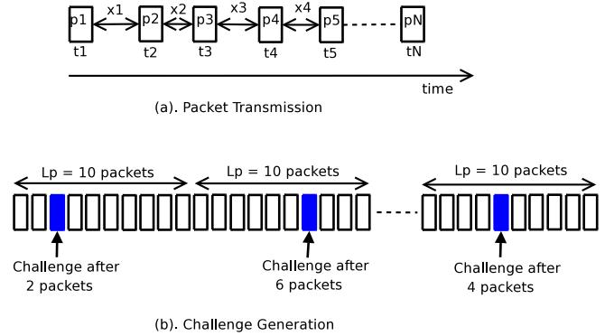
Figure 3: Data transfer scheme for location privacy preserving based routes (DTLPPR)
