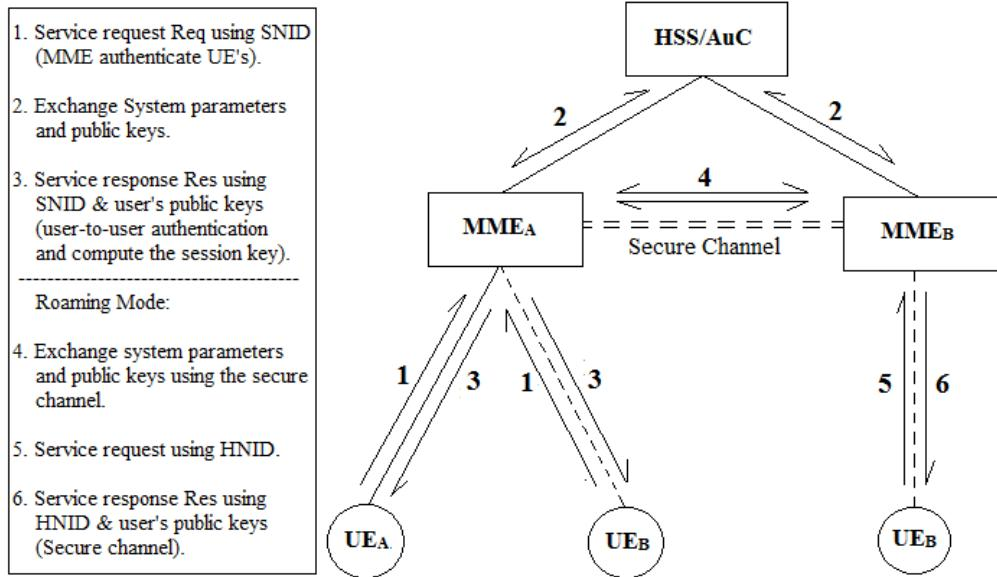
Figure 2: The proposed LTE-AKA handshaking process
