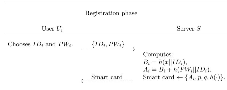
Figure 1: Registration phase of the proposed scheme
