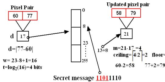
Figure 1: Data embedding through PVD with example
